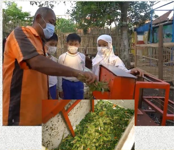
The process of cutting organic vegetable waste using a machine
