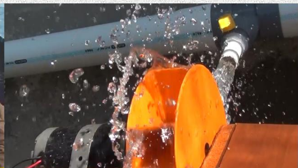
The turbine is driven by water flow. The turbine drives the generator
